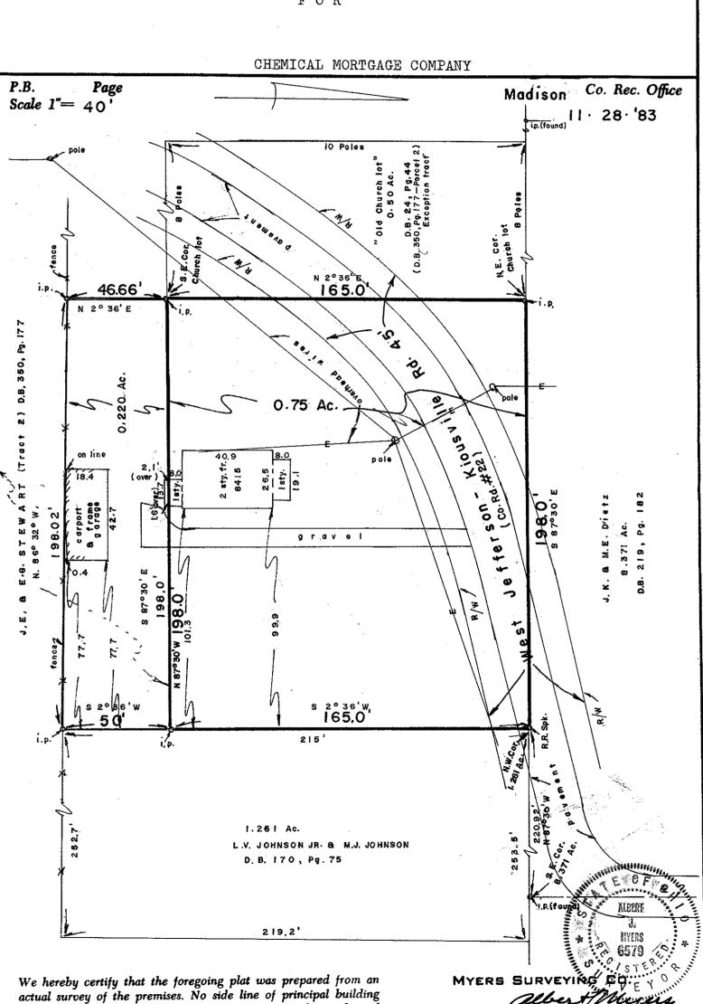
is less than dimension shown. Iron pins not set unless indicated thus -0- Iron pipes set are 30" X 1" O.D. with orange plug inscribed Applicant: HULLS "P.S. 3352". Bearing basis is from D.B. 170, Pg. 75
