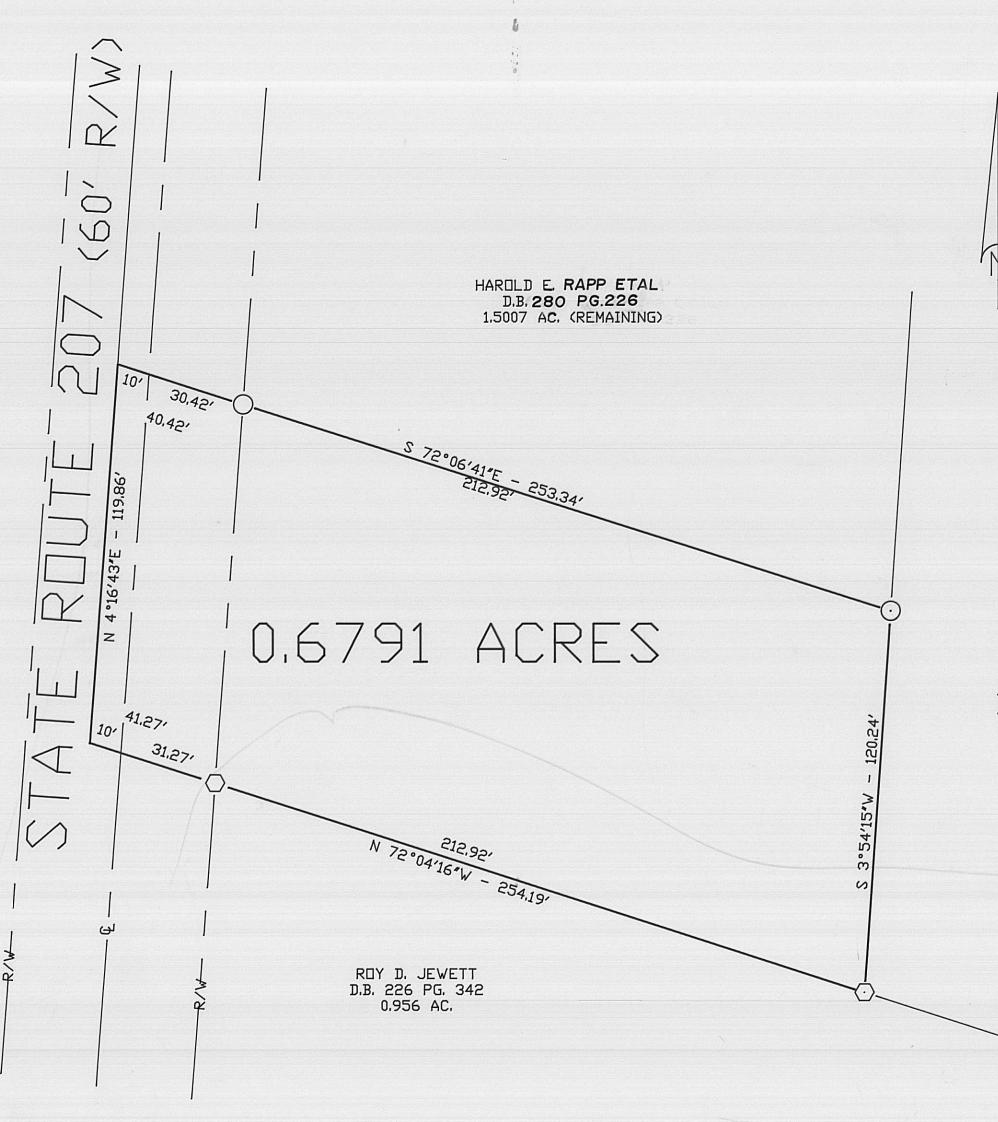
BEARINGS BASED ON THE SOUTH LINE OF RAPP'S 1.5007 AC. TRACTAS DESCRIBED IN D.B. 282 PG. 469. (S 72°06'41"E)
