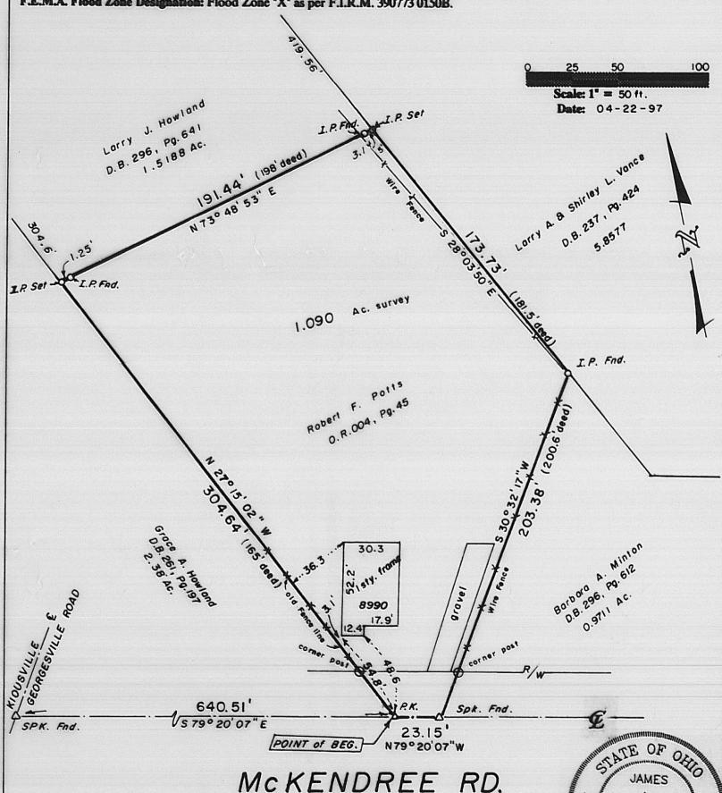
We hereby certify that the foregoing Boundary Survey was prepared from actual field measurements in accordance with Chapter 4733-37 Ohio Administrative Code. Iron pins set are 30"x1" O.D. with an orange plastic plug inscribed "P.S. 6579", unless otherwise noted. Basis of bearing is South 73 degrees 48 minutes 53 seconds West per a survey by James R. Cottrill, P.S. 6858, dated 8/23/93. D.B. 296, Pg. 641 - 1.5188 Ac. tract.
