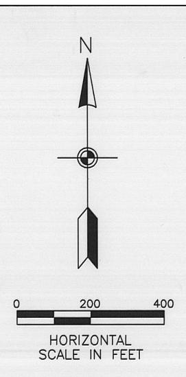
BEARINGS SHOWN HEREON ARE BASED ON THE CENTERLINE OF PLAIN CITY GEORGESVILLE ROAD BEARING SOUTH 06° 44' 00" EAST AS SHOWN IN INSTRUMENT NUMBER 200100000829, RECORDS OF THE RECORDER'S OFFICE, MADISON COUNTY, OHIO.
