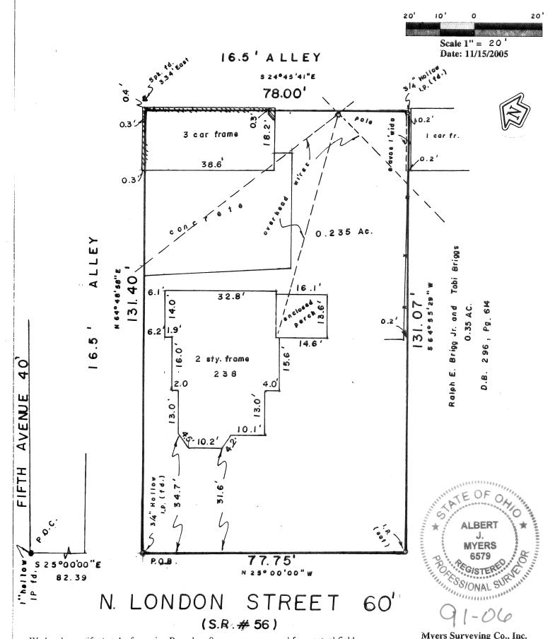
We hereby certify that the foregoing Boundary Survey was prepared from actual field measurements in accordance with Chapter 4733-37 Ohio Administrative Code. Iron pipes set are 30"x1" O.D. with an orange plastic plug inscribed "P.S. 6579", unless otherwise noted. Basis of bearings is the East Line of London Street as North 25 degrees 00 minutes 00 seconds West per Ins. 200500001709
