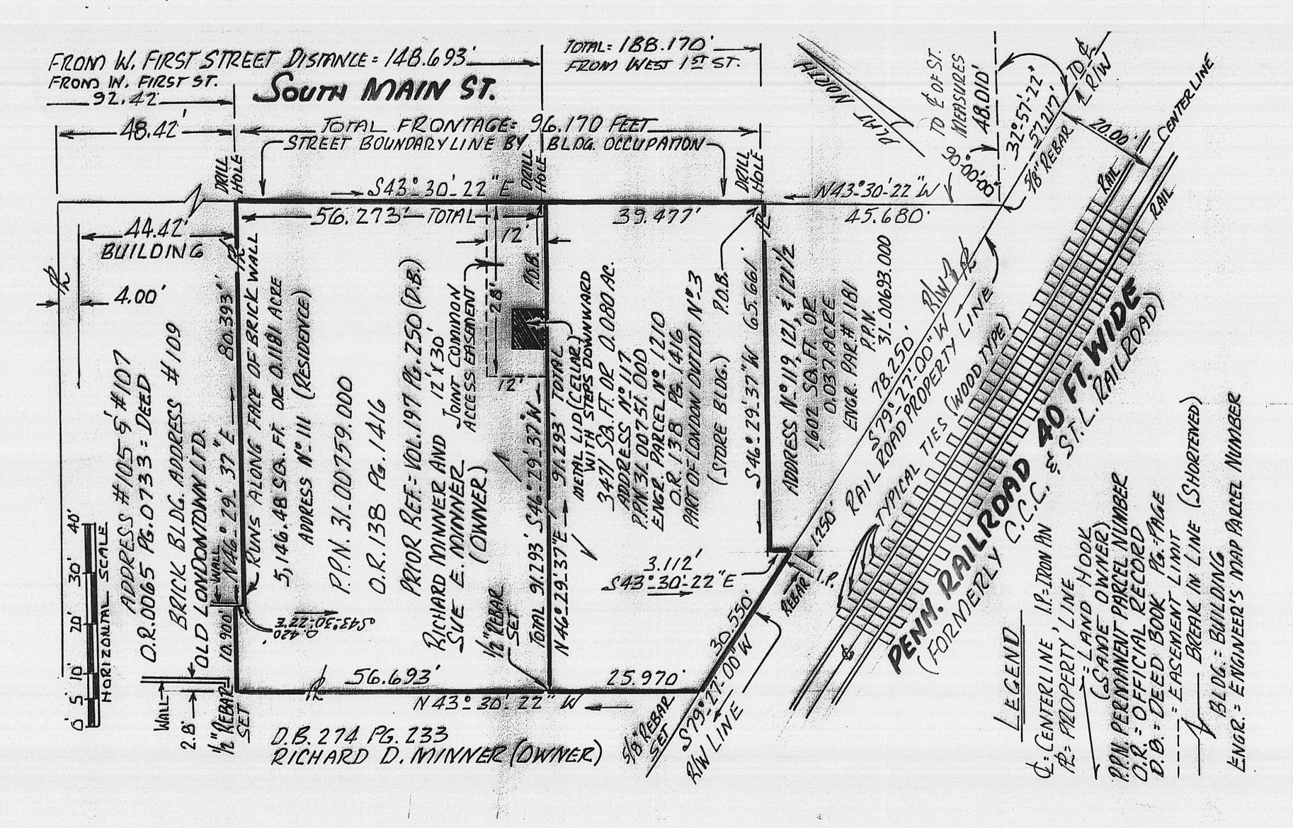
Bearings based on O.R. 138 Pg. 1416. Caps set on iron pins are stamped R.I.Baker S-5539.
