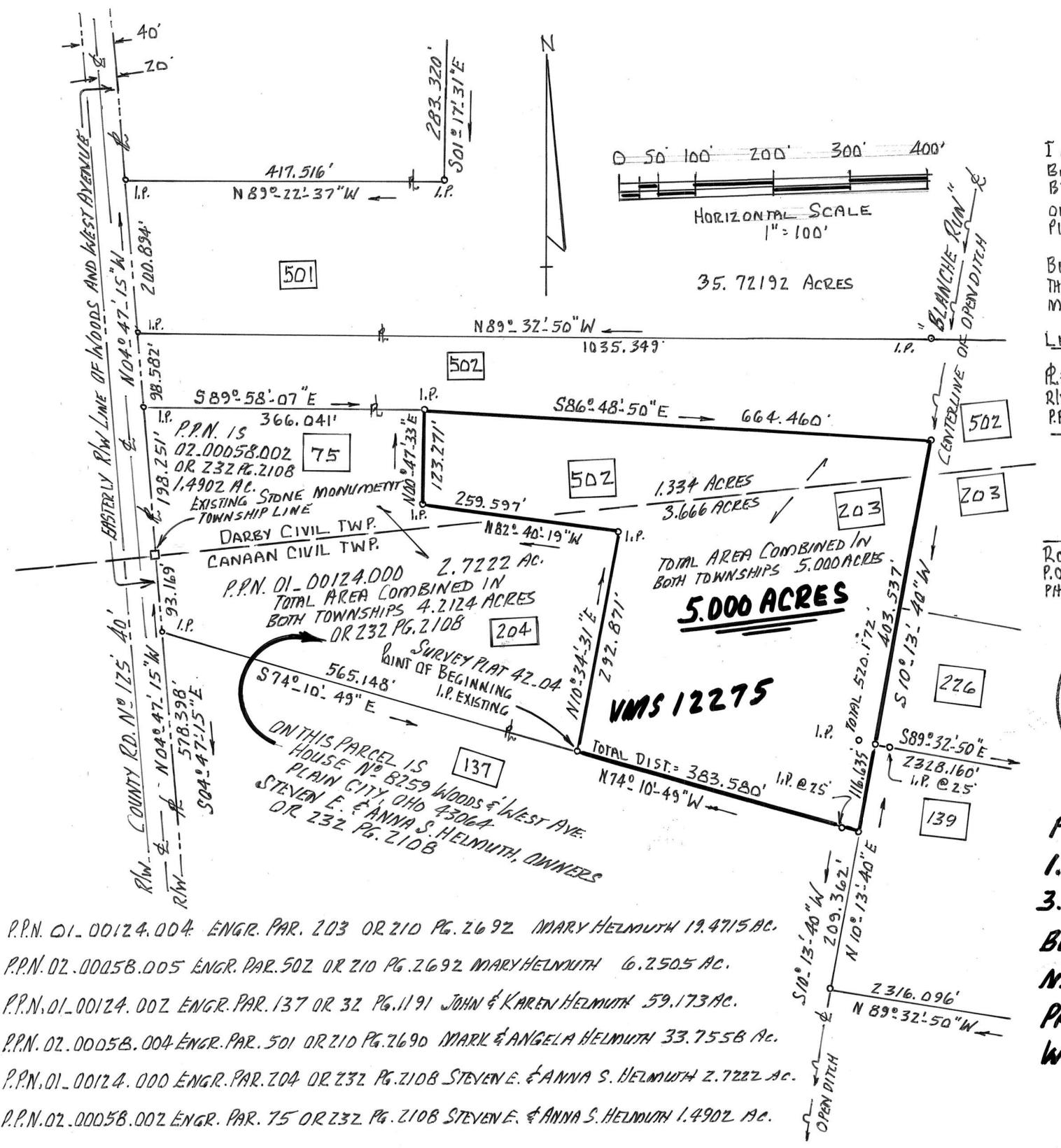
I CERTIFY THAT THIS PLAT HAS BEEN PREPARED BY ME AND IS BASED ON AN ACTUAL FIELD SURVEY MADE IN YEAR 2008 BY RODGER I. BAKER AND DILLON FOLLROD AS PER REQUEST OF JOHN HELMYTH AND OTHERS. PINS SET ARE REBAR WITTH PLASTIC CAPS STAMPED R.I.BAKER S.5539.
