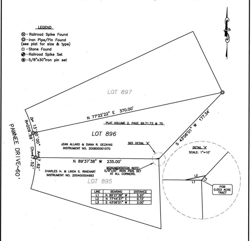
BASIS OF BEARINGS: ALL BEARINGS SHOWN ARE BASED ON THE OHIO STATE PLANE SYSTEM (NORTH ZONE) AS ESTABLISHED BY GPS OBSERVATIONS.
