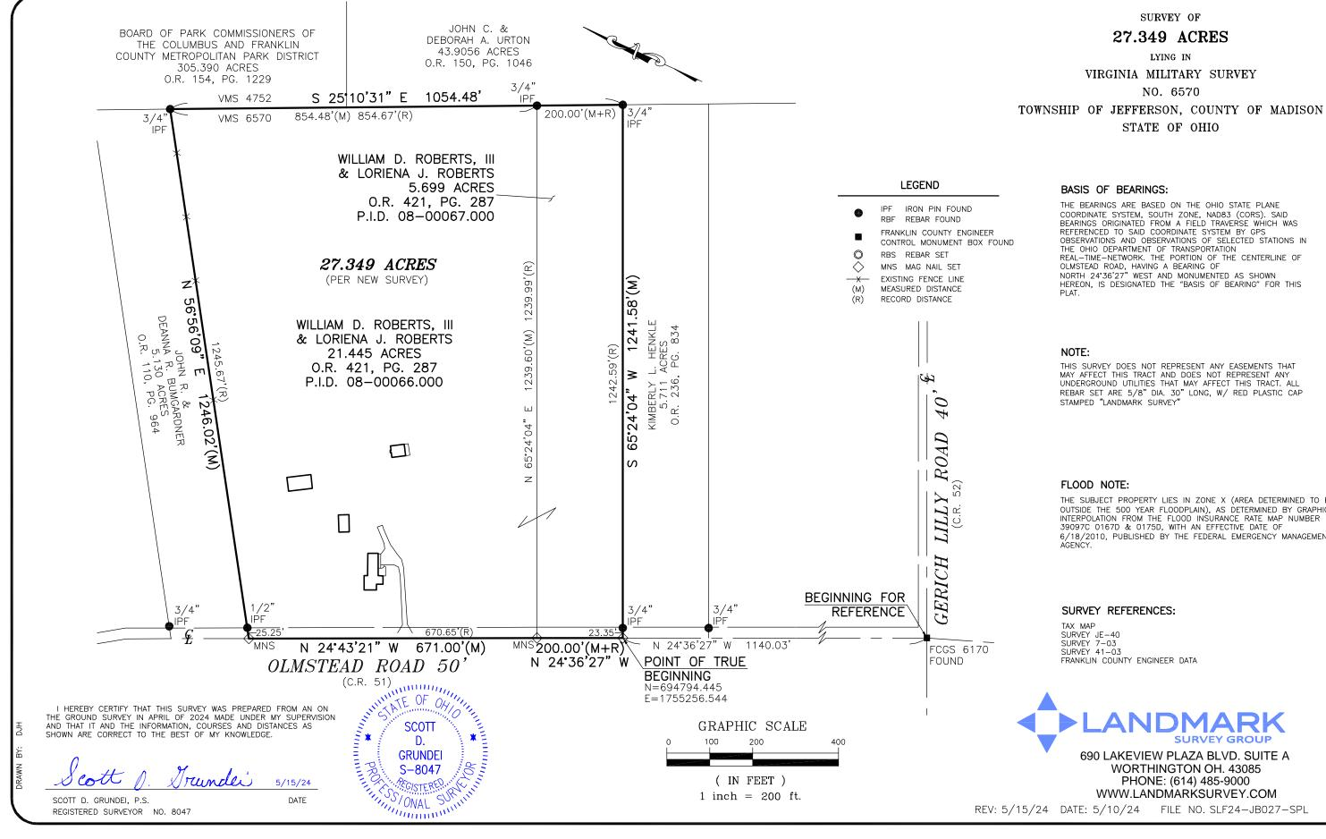
REFERENCED TO SAID COORDINATE SYSTEM BY GPS OBSERVATIONS AND OBSERVATIONS OF SELECTED STATIONS IN REAL-TIME-NETWORK. THE PORTION OF THE CENTERLINE OF OLMSTEAD ROAD, HAVING A BEARING OF NORTH 24'36'27" WEST AND MONUMENTED AS SHOWN HEREON, IS DESIGNATED THE "BASIS OF BEARING" FOR THIS
