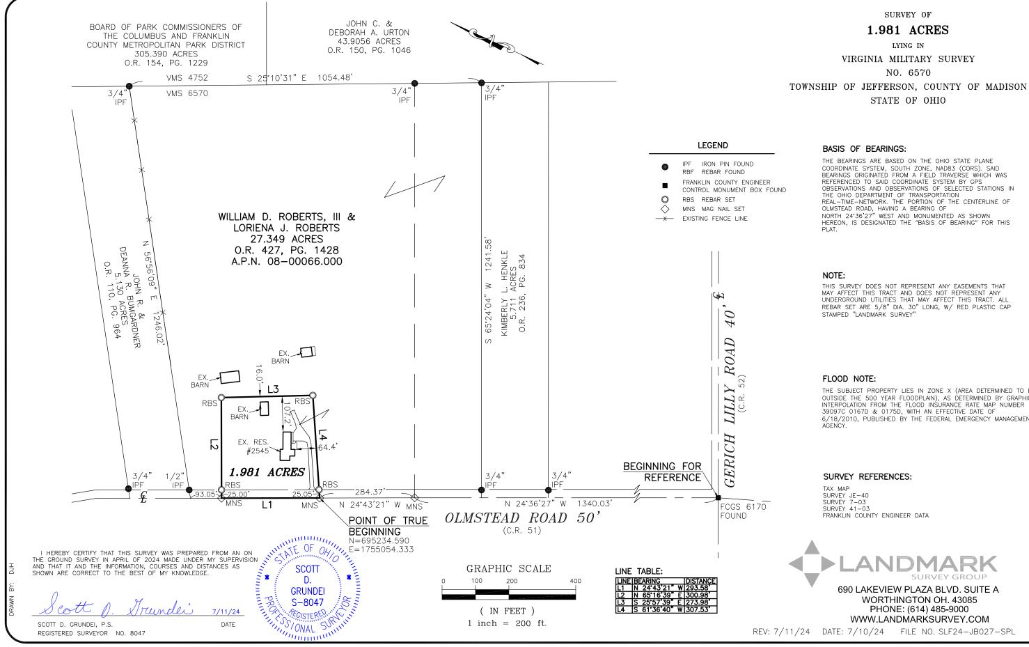
BEARINGS ORIGINATED FROM A FIELD TRAVERSE WHICH WAS REFERENCED TO SAID COORDINATE SYSTEM BY GPS OBSERVATIONS AND OBSERVATIONS OF SELECTED STATIONS IN REAL-TIME-NETWORK. THE PORTION OF THE CENTERLINE OF OLMSTEAD ROAD, HAVING A BEARING OF NORTH 24'36'27" WEST AND MONUMENTED AS SHOWN HEREON, IS DESIGNATED THE "BASIS OF BEARING" FOR THIS
