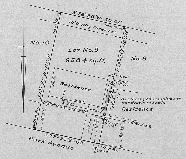
Icertify all dimensions on the above Plat are correct, Iron Pin were set as shown and one encroachment found.
